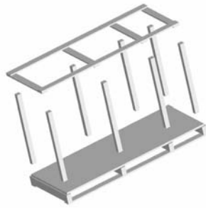
Internal packaging structure with cardboard walls;
